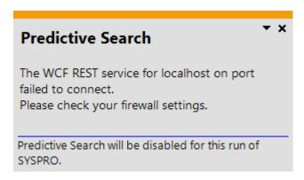
This message indicates that the REST port in the **Setup Options** program has not been configured, or is not configured correctly.
