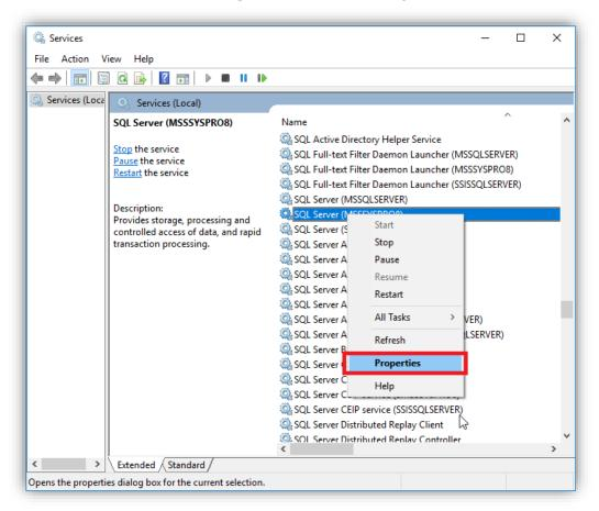
Under the General tab you can see the Service name. In this case: MSSQL\$MSSSYSPRO8
