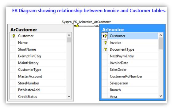
Figure 4 Simple Entity Relationship Diagram
